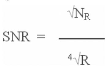
where  $N_R$  is the reconstructed counts per pixel and R is the number of pixels (resolution elements) containing activity ( $_5$ ). Thus, using an eight interval gated SPECT, a 64 x 64 matrix, a ramp filter and assuming no beat rejections, the reconstructed SNR will deteriorate by a factor of 2.83 for gated data (over the ungated data).
