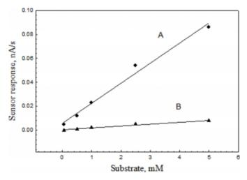
By contrast, Fig. 2 shows the calibration dependence of a microbial sensor based on B. subtilis strain VKM B-434 for sucrose and maltose. Although the kinetics are more complex in this case, practical response ranges were determined to be 0.05-5.0 mM for maltose and 0.005-0.5 mM for sucrose. Clearly, this sensor responds more strongly to sucrose.
