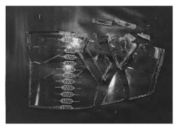
Test 3: Within seconds of coming into contact with either of the two anesthetics, visible cracks formed in the venous
