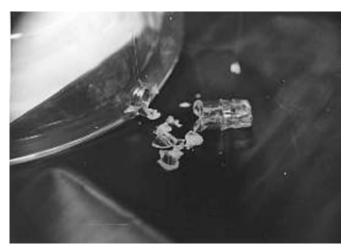
Test 4: The base of the venous reservoir of all the used and the new oxygenators cracked.
