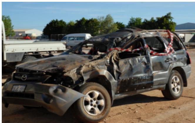
Fig. 5: Main cab intact over driver and passenger
