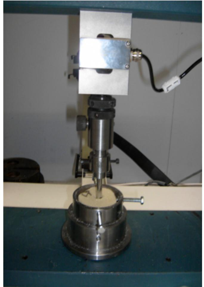
Custom designed jigs (Figure 1.) were used to secure both the implants and the test specimens ensuring that the only movement that would occur during testing would be at the interface between the implant and the test material.
