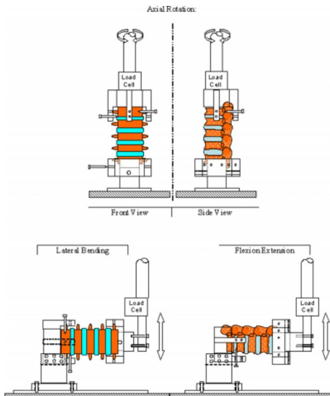
Diagram illustrating the methods and modes of testing the specimens using the Instron machine.
