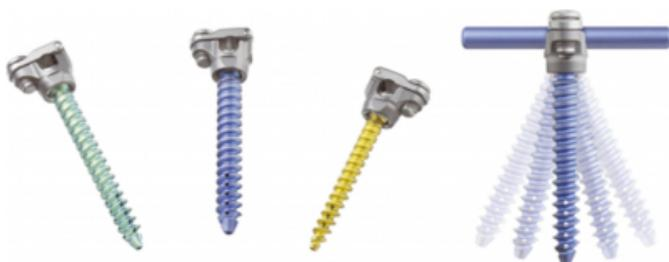
The screws are perforated in the anterior third of the thread to allow screw augmentation with bone cement after inserting the screw. Due to a special augmentation adapter, which is temporarily fixed to the screw, there is no risk of cement leakage blocking the polyaxial mechanism after augmentation {Figure 2}. A special reduction instrument allows easy reduction of a spondylolisthesis of up to 50%.
